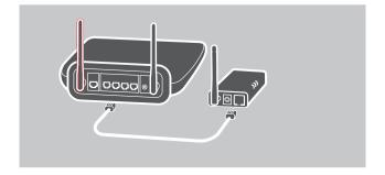
3. Plug one end of the power adapter to the Print Server and the other into an electrical outlet. The Print Server will perform a Power-On Self-Test (POST) after it is powered on. When the Status LED light goes off, the Print Server is ready.
